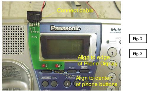
6- Connect the Sensor Cable to the Sensor Board.
