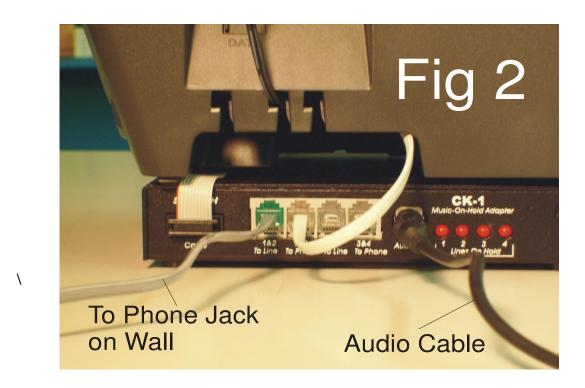
3- Connect the audio cord from your audio source, to the AUDIO IN jack on the back of the CK-1 box. For DIGITAL, USB, or MP3 players, use the cable that comes with the player, not ours. Our cable is for CD players ONLY. For DIGITAL, USB, or MP3 players, the ends of the cable will have the same type of connector (RCA). (Fig 2)
