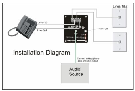
When a line is placed "ON HOLD", the corresponding LED on the AS-703-M will light indicating that audio is being coupled to that telephone line. The unit will play audio to all calls that are placed ON HOLD. Make sure that you adjust the level of the music to the proper level on the audio source.
