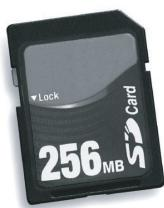
The player is also equipped with a slot for a Secure Digital (SD) flash card. Files can be copied to the card by putting it into the unit and connecting the USB cable to a PC. Alternately, files can be copied to the card by connecting a smart media card reader to the PC's USB port and copying files directly to the card.
