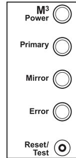
The **Reset/Test** button is used to mute the audible alarm if a failure or error occurs. Additionally, during normal operation, you may test the M3 panel indicators by pressing and holding **Reset/Test** for more than one second. This will turn on all of the M3's LEDs and sound the audible alarm until you release the **Reset/Test** button.
