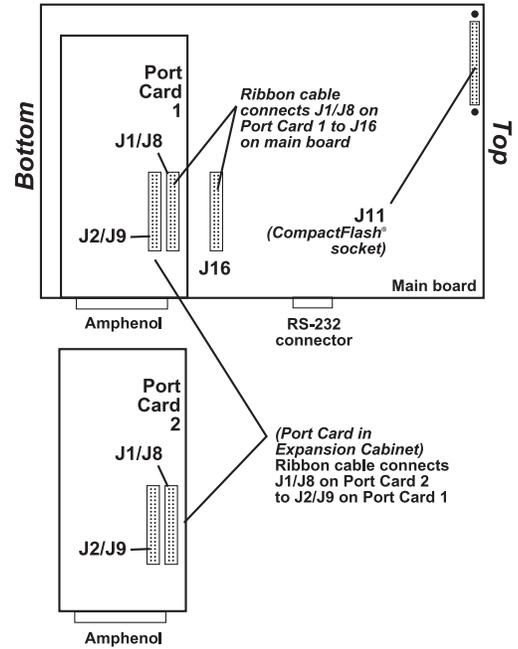
The diagram at *right* shows the configuration of a fully loaded ESI-50.
