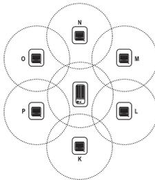
Repeaters that are registered directly to a base station (*left*), do **not** require use of the optional **Repeater Configurator Kit**. These Repeaters can be installed using automatic configuration. However, Repeaters registered to the base station **through** another Repeater (one example shown, *right*) **do** require use of the Repeater Configurator Kit.
